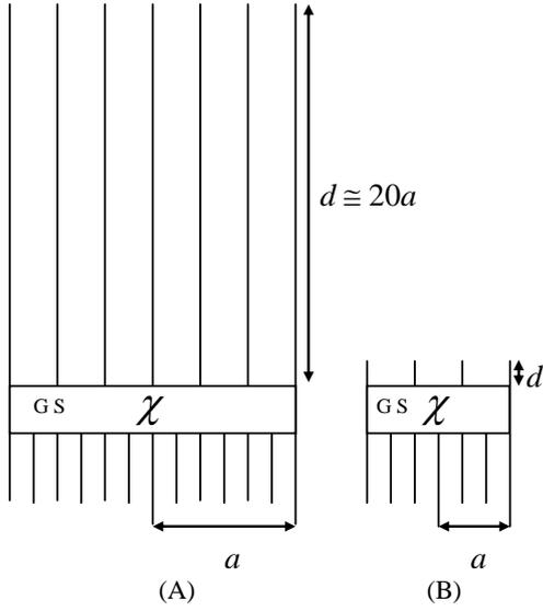
Fig. 4 - When the shielding's surface is large the action of the gravitational shielding extends up to a distance  $d \cong 20a$  (A). When the shielding's surface is *very small* the extension of the shielding effect becomes experimentally undetectable (B).
