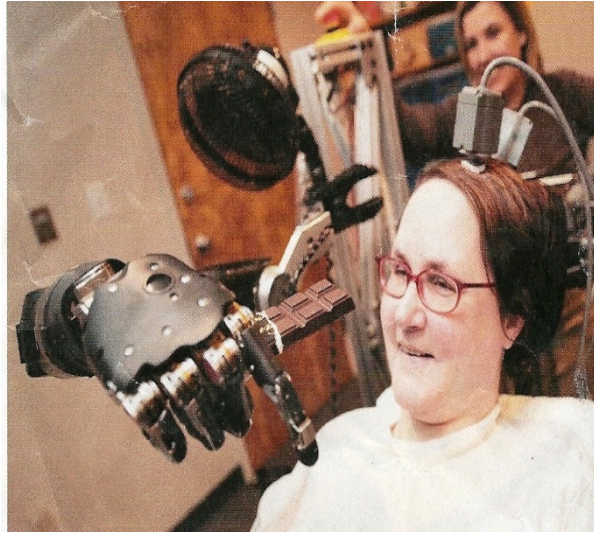
Figure 2a. Brain-controlled Mechanical Arm and Hand [44[26]], Reardon, 2014.
