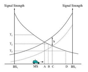
Fig. 1. Signal strength and hysteresis between two adjacent BSs for potential handoff [17].
