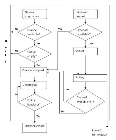
Fig. 2. Call Flow Diagram for the Measurement Based Prioritization Scheme [21].
