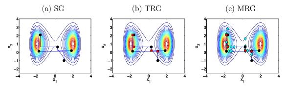
Figure 5: We consider T=4 iterations of a Gibbs sampler and M=5 iterations of the MH for drawing from each full-conditional pdfs. (a) With the circles we denote the T+1 points (considering the starting point) used in the standard Gibbs estimators. (b) The vectors (denoted with circles and squares) used in the TRG estimators. (c) The vectors (denoted with circles, squares and diamonds) used in the MRG estimators.
