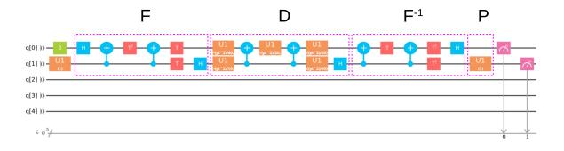
FIG. 1: The two-qubit quantum circuit for one time step simulation. The quantum circuits for the kinetic  $(FDF^{-1})$  and potential (P) energy operators are depicted.
