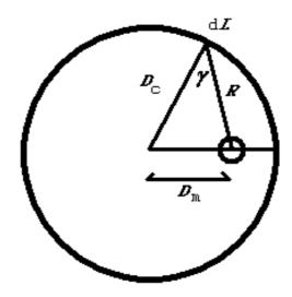
Figure 1: Diagram showing the symbols used when the small, round magnet is in a solenoid.
