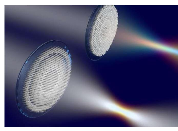
Illustration showing a comparison between two types of flat lenses. In the foreground, a new type of flat lens focuses all colors of light to the same spot. As a comparison, the flat lens in the background is not color-corrected. Credit: Adam Overvig/ Columbia Engineering
