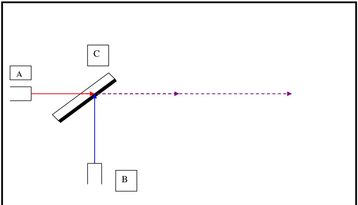
An electromagnetic wave source A generates the very focused first (red) one dimensional electromagnetic traveling wave , which passes through the half transparent mirror C, and is supposed to continue, after it passes the half transparent mirror C (as the dotted line indicates).
