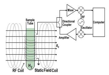
**Fig.17.** Simplified experimental NMR-like resonance apparatus for putative LSXD C-QED ionization of TBS in hydrogen. The Fig. only shows possible details for rf-modulating TBS QED resonance, not the spectrographic recording and analysis components.
