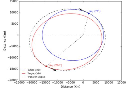
Fig. 4: Analytically generated transfer ellipse
