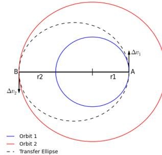
Fig. 1: Hohmann transfer example.
