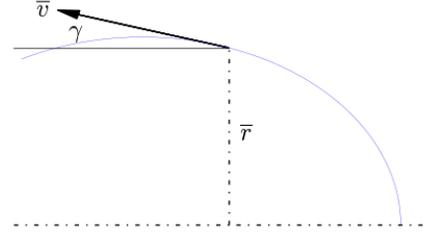
Fig. 3: Flight Path Angle ( $\gamma$ )
